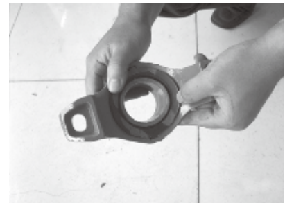
3. Put gasket seal in the Mechanical Tee.
